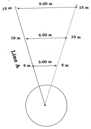
As an aid in marking and checking the 34.92 degree sector lines, the table below may be used (for greater accuracy, use the longest distance your field will allow and work toward the circle in laying out your marks for line B). In this table, A indicates the distance from the center point of the circle to a point on each of the two sector lines and B indicates the distance between those two points. A **metric measurement** will make it more accurate.
